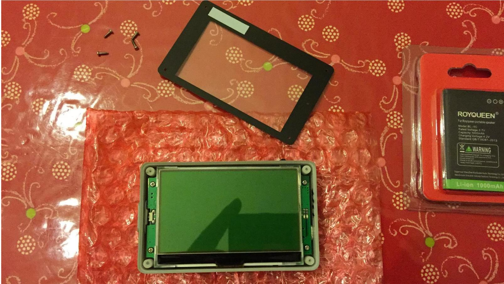
Disassembly step 3: unscrew remove the screws from PCB
