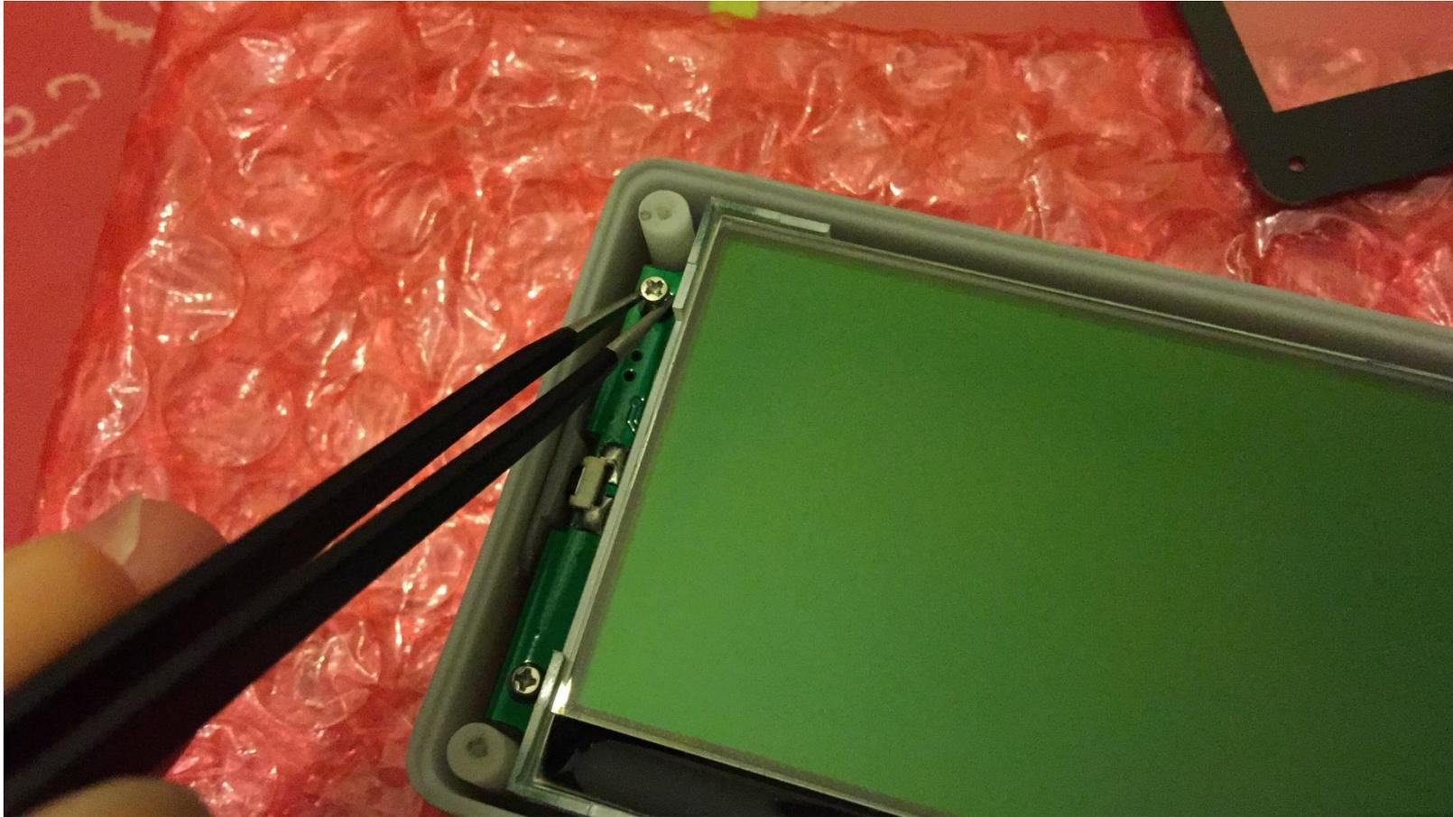
Disassembly step 4: remove the PCB
