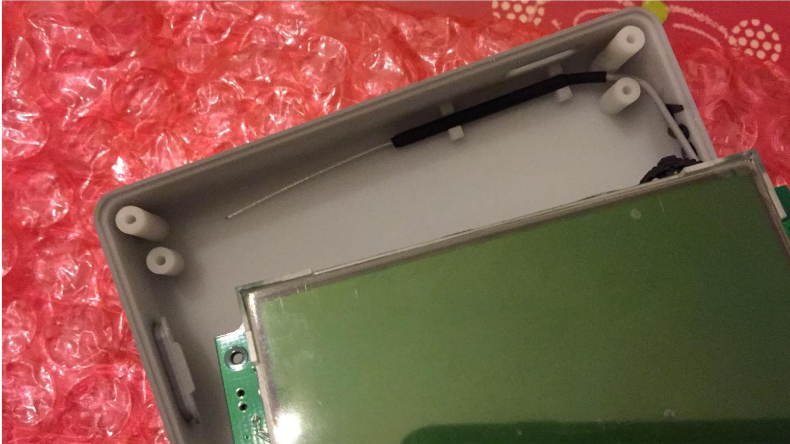
Tear off the protect film of the LCD
