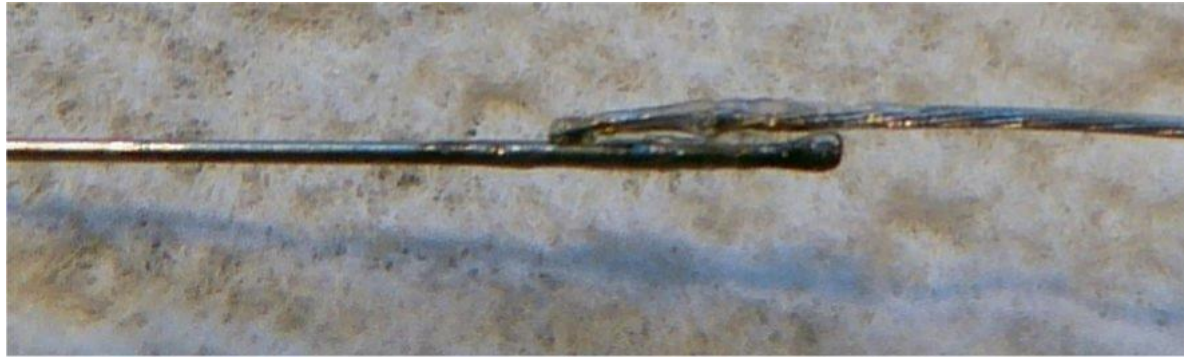
P13 Join 0.3 wire to cable.jpg (44.97 KB, 923x265 - viewed 45 times.)
