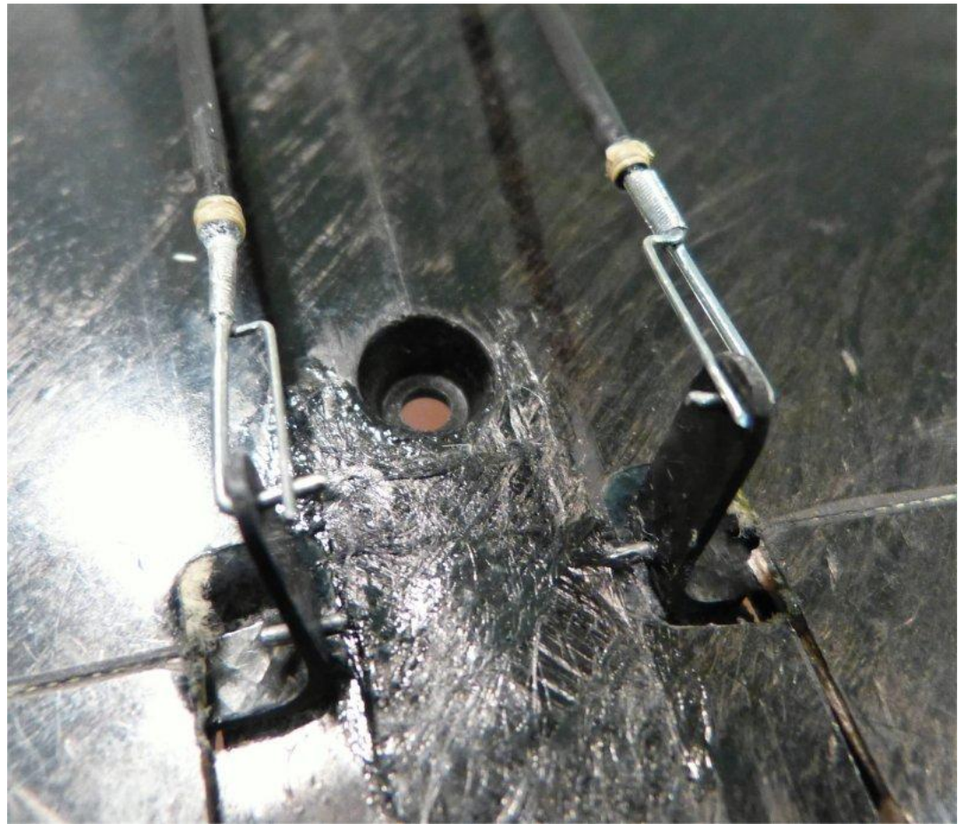
5 Flapperon horns with rods.jpg (112.31 KB, 800x691 - viewed 29 times.)
