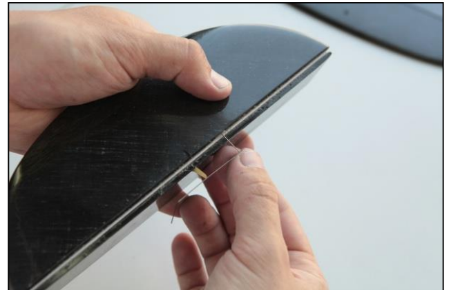
Figure 2.5 - Insert the torsion bar in the tail
