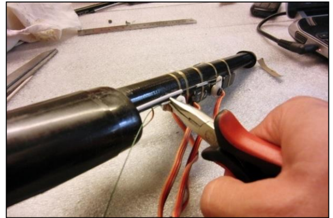
Figure 2:31 – Crimping of tube for tail control
