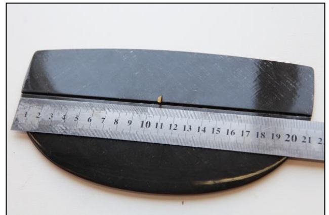
Figure 2.2 – rudder horn installation location
