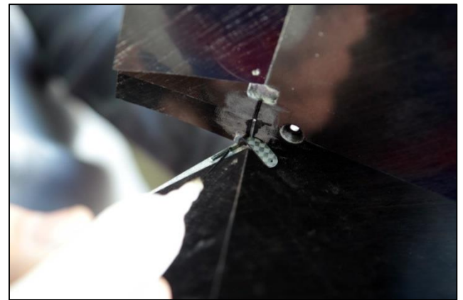
Figure 2.22 - Bonding horn inside the aileron
