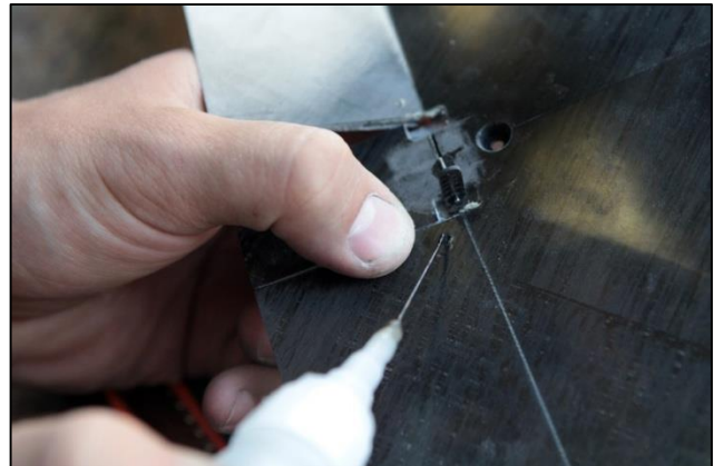
Figure 2.20 - Bonding horns thick CA through the hole in the aileron
