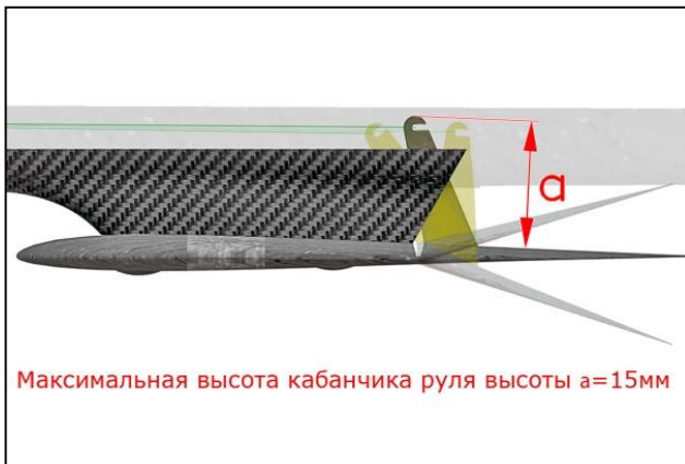
Figure 2.3 - Maximum elevator horn length
