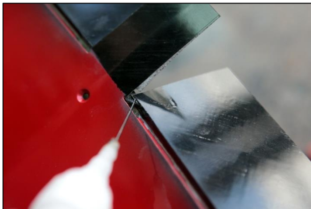
Figure 2.21 - Bonding horn inside the aileron
