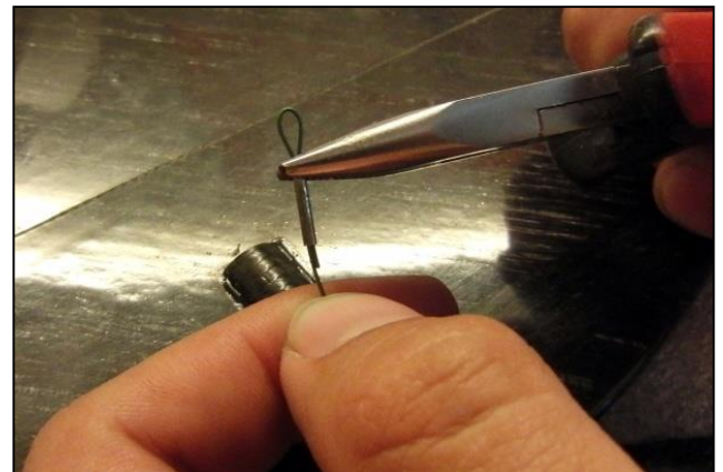
Figure 2.11 - Crimping tube cable
