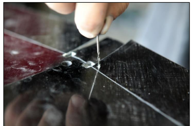
Figure 2.17 - Holes for gluing horn in flaperon
