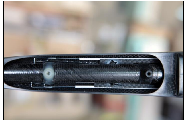
Figure 2.39 - Fixing the aileron linkage inside the fairing
